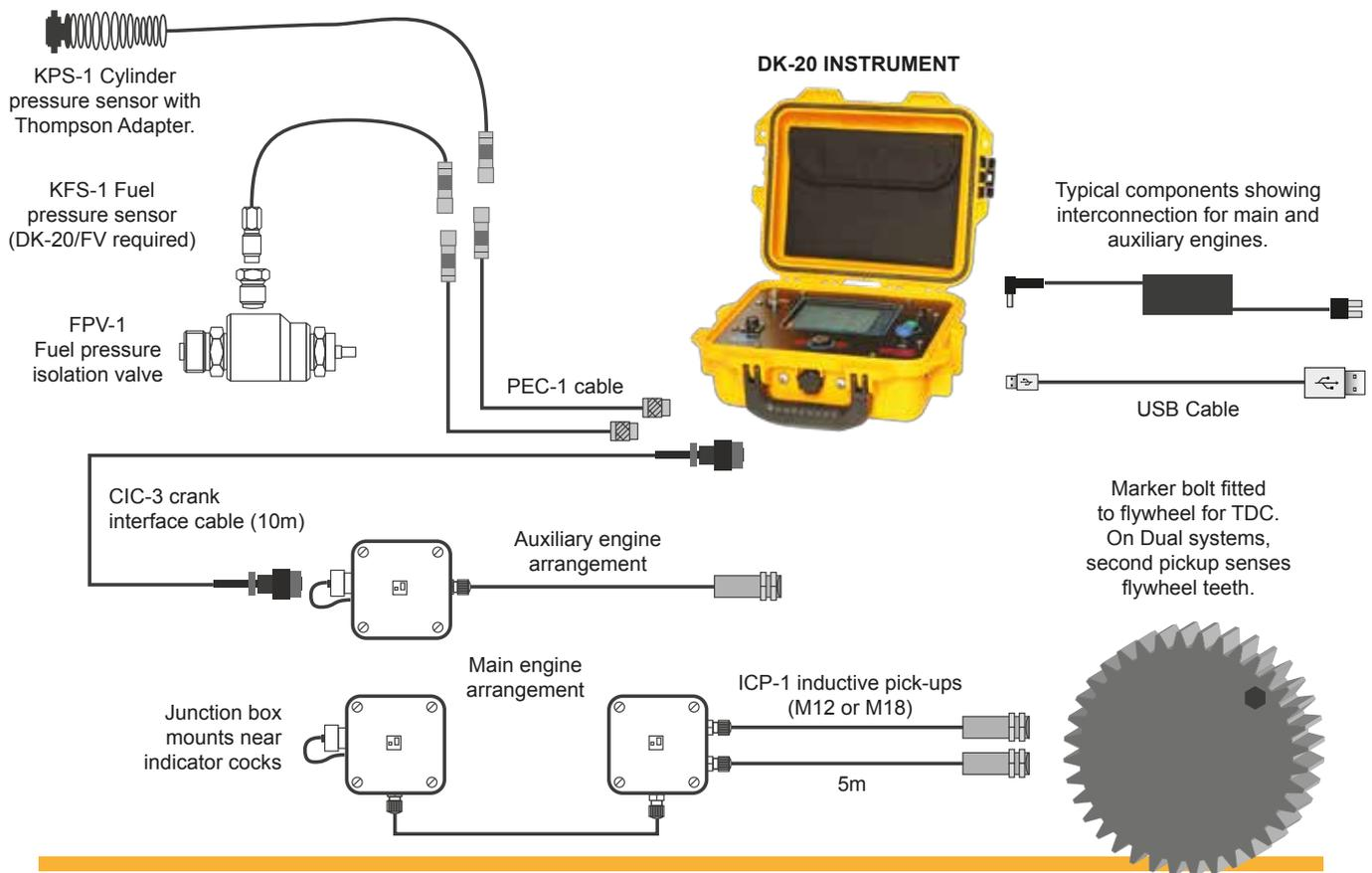
The Doctor instrument is available in two versions, namely the single channel DK-20 for cylinder pressure only measurements, and the two channel DK-20/FV which incorporates a second channel for simultaneous fuel or vibration measurement.
